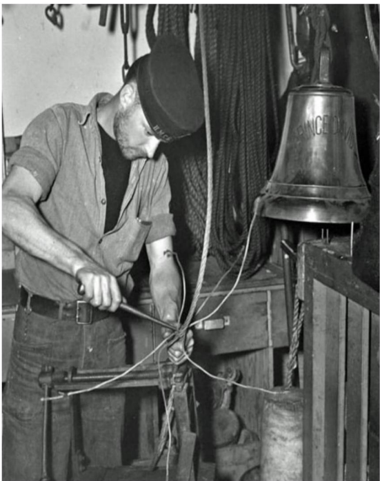
AB Murray Kennedy splicing cable aboard H.M.C.S. PRINCE DAVID, Cowes, England, 10 May 1944. Submitted by William Gard.
